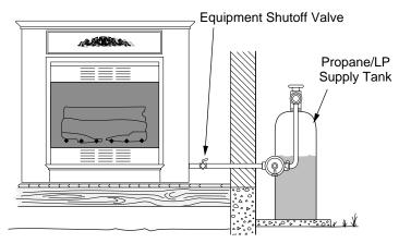
Figure 26 - Checking Gas Joints for Propane/LP Units (Shown with Optional Mantel)
